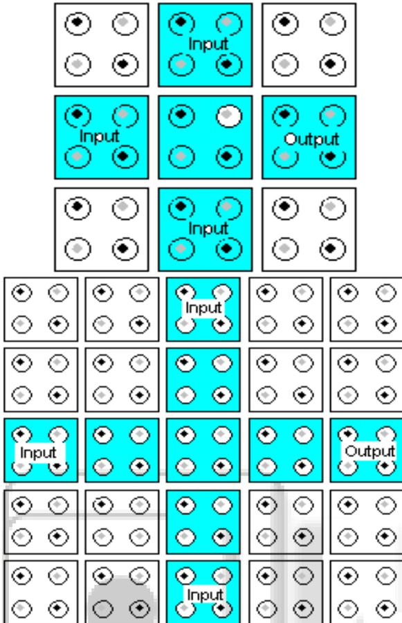
Fig. 2.1: 3X3, 4X4 QCA tile based block for a majority logic
