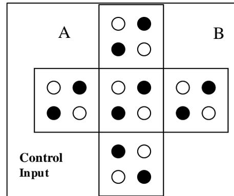
Fig. 1.2: QCA Majority AND gate. Control input is -1.
