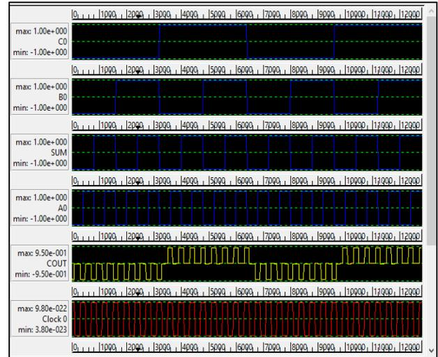
Fig. 3.2: Simulated waveform of QCA Full adder
