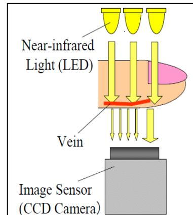
Fig. 2.1.1: Light Transmission Method
