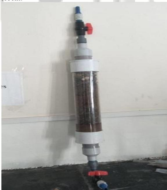
Fig. 1: Low cost water purification setup
