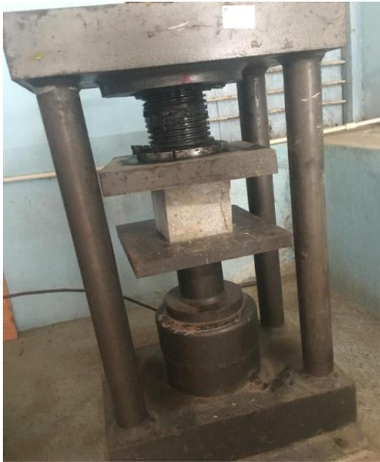
Fig. 1: Compression test on concrete
