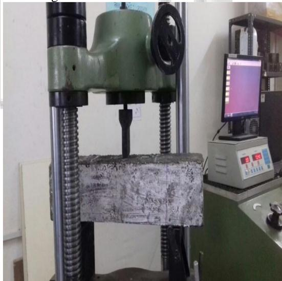
Fig. 2: Flexural test on concrete
