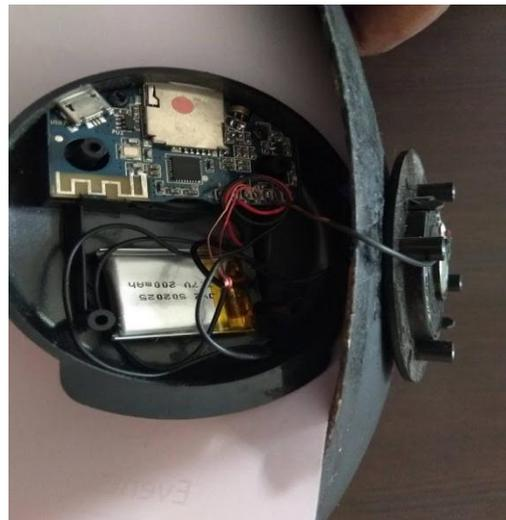
Fig. 3: Bluetooth Module Powered by LIPO Battery
