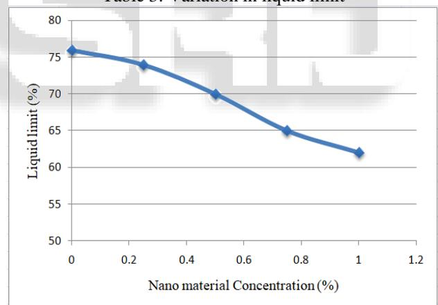
Fig. 3: Variation of liquid limit with nano content
