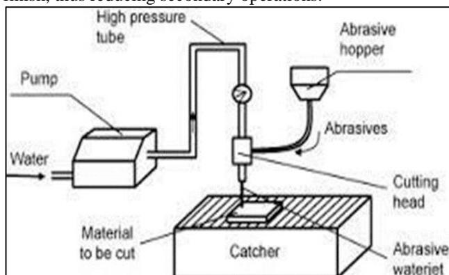
Fig. 1: Abrasive Water jet machine Setup
