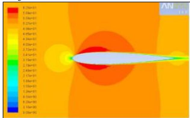
Fig. 9: Velocity contour of NACA 0012 at zero AOA
