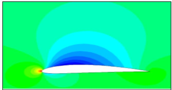
Fig. 6: Pressure contour of NACA 4412 at zero AOA
