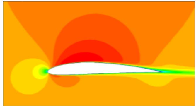
Fig. 7: Velocity contour of NACA 4412 at zero AOA
