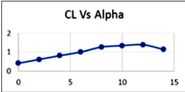
Fig. 10:  $C_l$  vs Alpha Curve for NACA 4412
