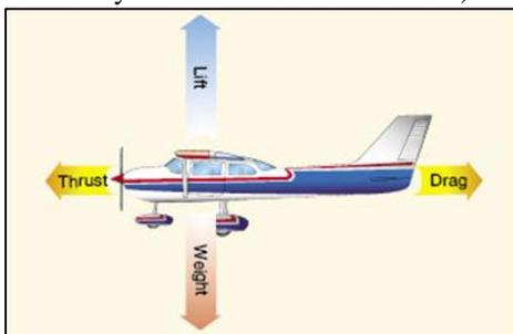
Fig. 1: Forces acting on an airplane
