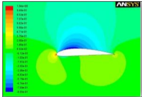
Fig. 12: Pressure contour of NACA 4412 at zero AOA
