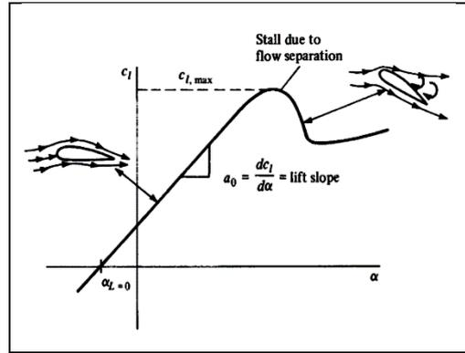
Fig. 4: Lift Coefficient variation with angle of attack for cambered airfoil
