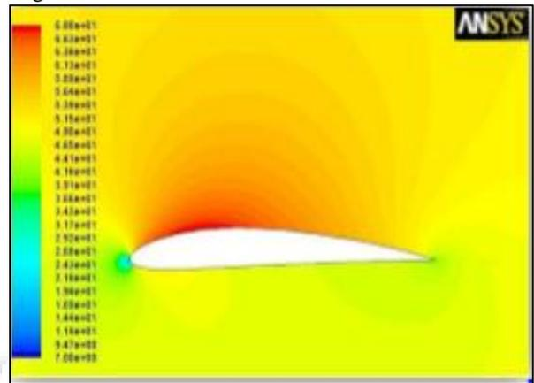
Fig. 13: Velocity contour of NACA 4412 at zero AOA
