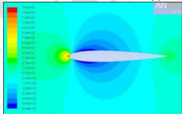
Fig. 8: Pressure contour of NACA 0012 at zero AOA
