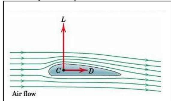
Fig. 2: Lift and Drag over an Airfoil
