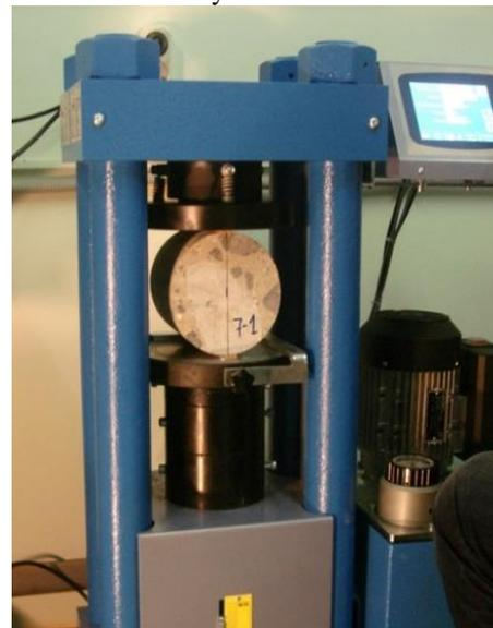
Fig. 4: Split tensile test on cylinder
