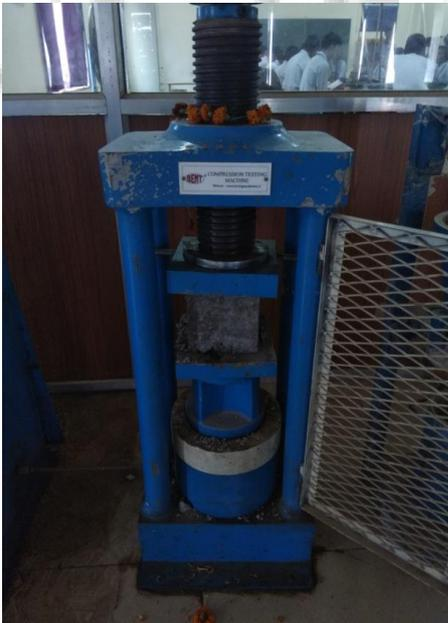
Fig. 2: Compression test on Cube
