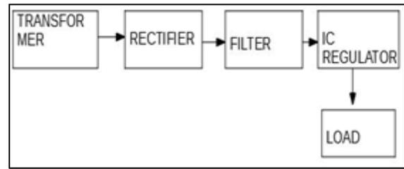
Fig. 2: Block Diagram of Power supply
