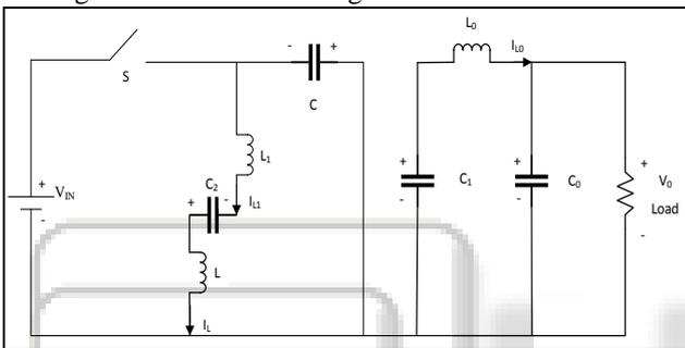
Fig. 8: Equivalent circuit when switch S is OFF state
