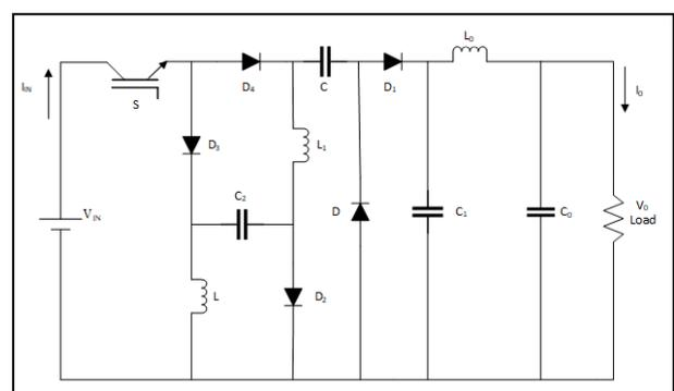
Fig. 6: Circuit diagram of Luo converter
