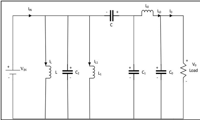
Fig. 7: Equivalent circuit when switch s is in ON state
