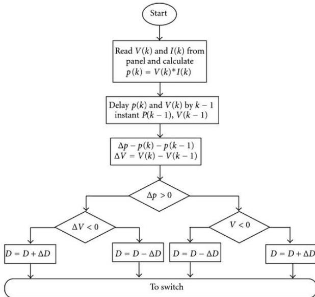
Fig. 3: Flow chart of P&O MPPT algorithm
