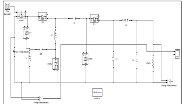
Fig. 5: Simulation of Luo converter
