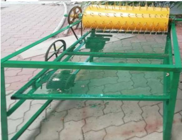
Fig. 5: Prototype Model of grain separator
