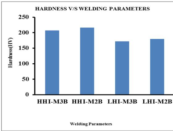
Fig. 8: Graph between hardness and welding parameters
