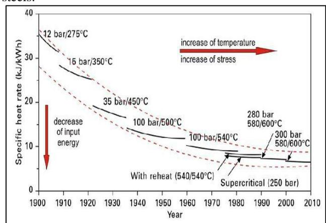
Fig. 1: Stages of development of material for higher temperature application
