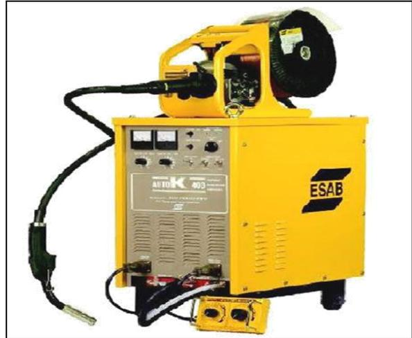
Fig. 2: Welding machine (GMAW, ESAB AUTO K 400)
