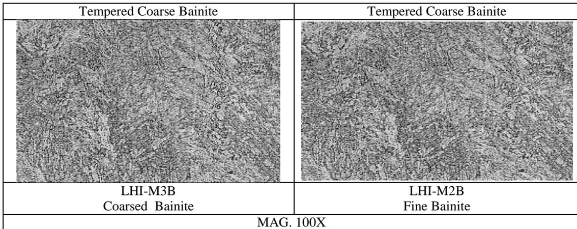
Fig. 10: Microstructure of weld metals
