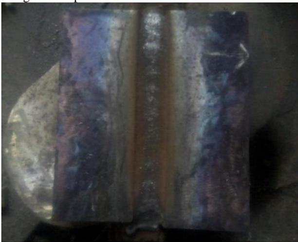
Fig. 3: HHI-M3B weld joint
