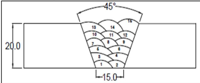
Fig. 5: Low heat input weld joint
