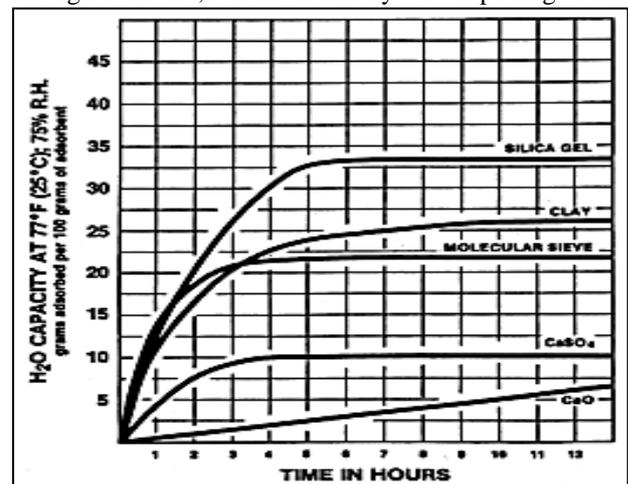
Fig. 3: Adsorption rate of various adsorbents
