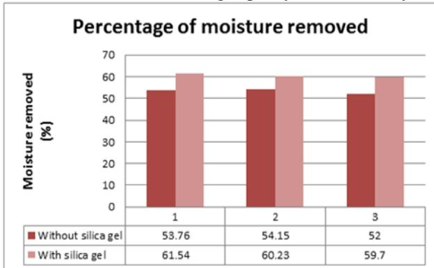
As seen from the above column chart, percentage of moisture removed is more when silica gel is employed. On an average, 7% more moisture is removed by incorporating silica gel.
