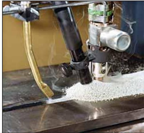
Fig. 1: Submerged Arc Welding
