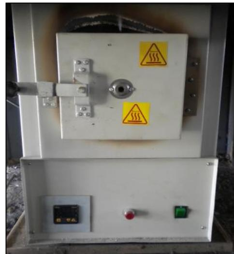
Fig. 2: Furnaces for Baking Flux
