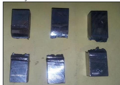
Fig. 3: Specimens after Impact Testing
