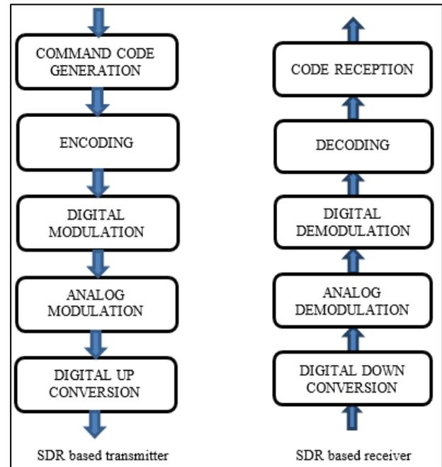
Fig. 3: SDR based transmitter and receiver
