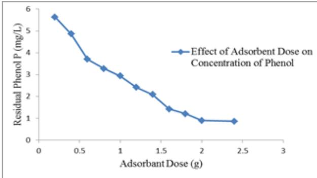
Fig. 02: Effect of Saw Dust (Dose) on Adsorption of Phenol
