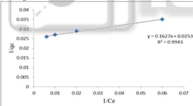
Fig. 04: Langmuir Isotherm plot of Phenol-Sawdust adsorption System
