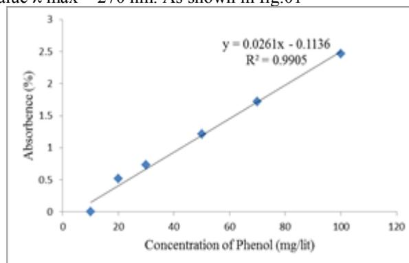
Fig. 01: Calibration graph for Phenol Concentration with % Absorbance
