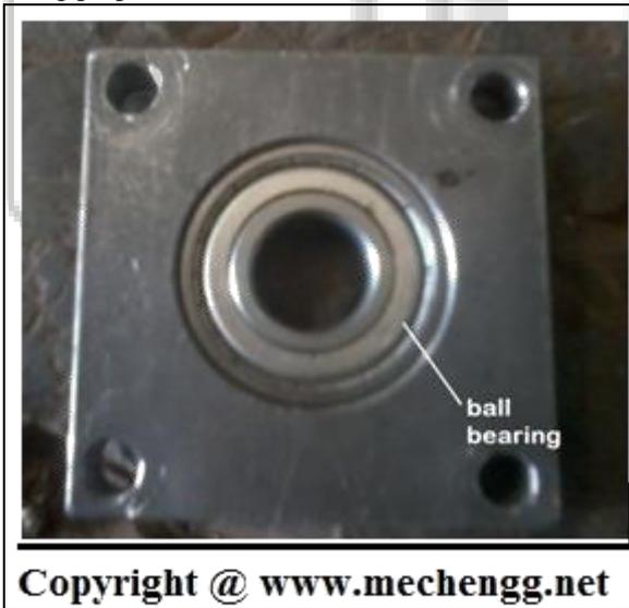
Fig. 3: Bearing Mounter Plate
