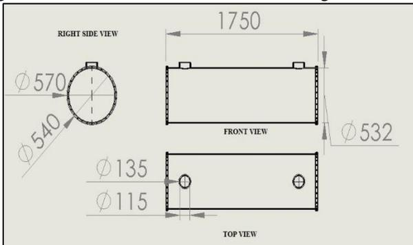
Fig. 1: 2-D Front view, Top view and Right side view of Shell
