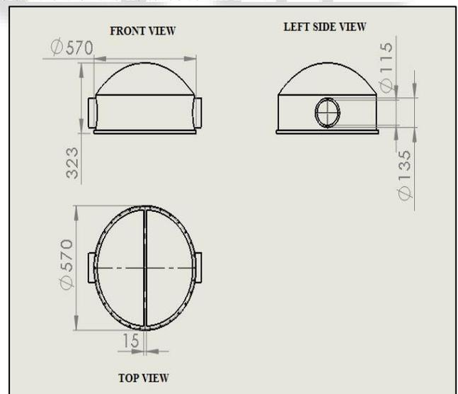
Fig. 5: 2-D Front view, Top view and Left side view of the head cover
