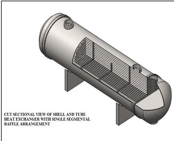
Fig. 6: Cut-sectional view of modelled shell and tube heat exchanger with single segmental baffle arrangement
