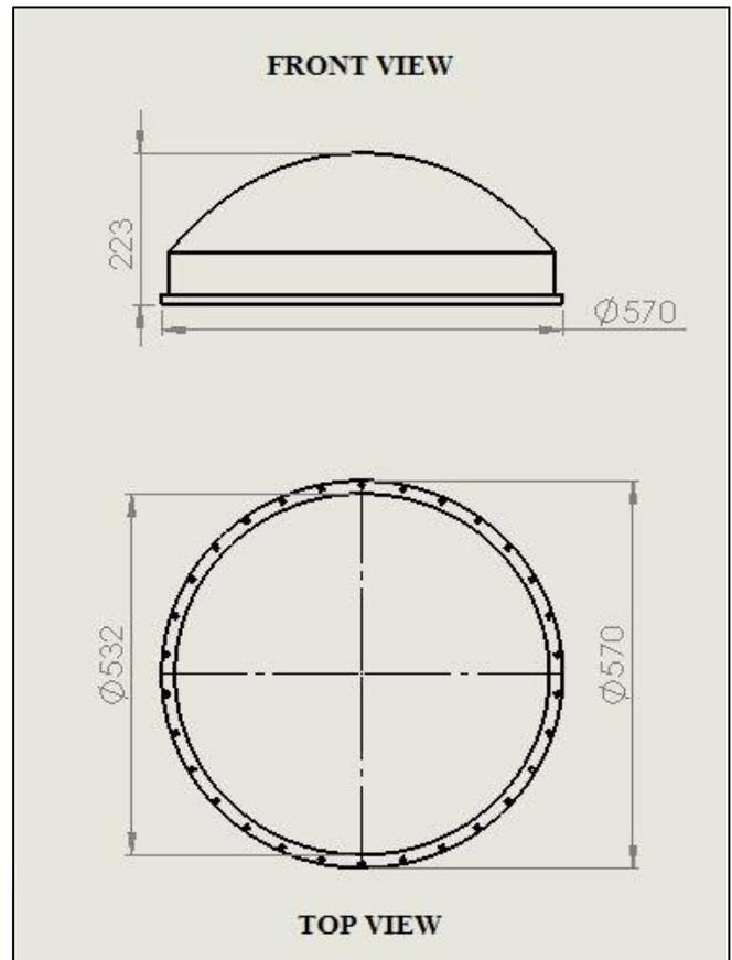
Fig. 4: 2-D Front View and Top View of the Shell cover
