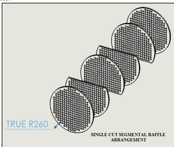
Fig. 3: Single cut segmental baffle arrangement with tube sheets
