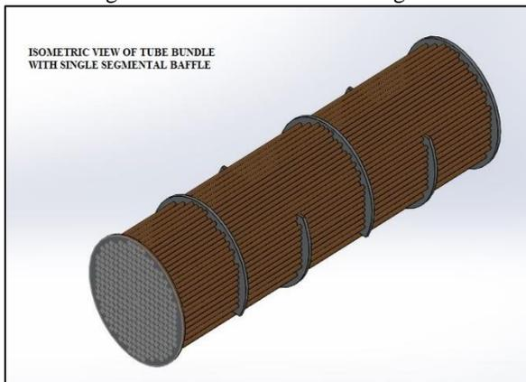
Fig. 2: Isometric view of tube bundle with single segmental baffle
