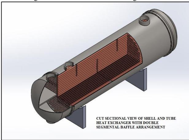
Fig. 7: Cut-sectional view of modelled shell and tube heat exchanger with double segmental baffle arrangement
