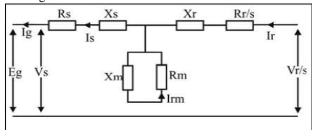
Fig. 1: Equivalent circuit of doubly fed induction generator
