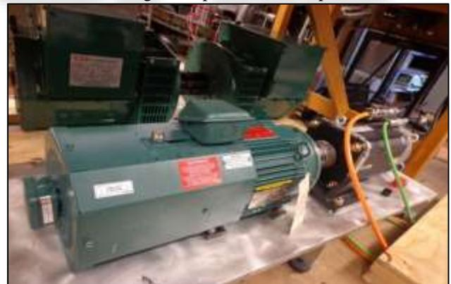
Fig. 3: PMSG coupled with a DC generator
