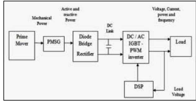
Fig. 1: Schematic of WECS
