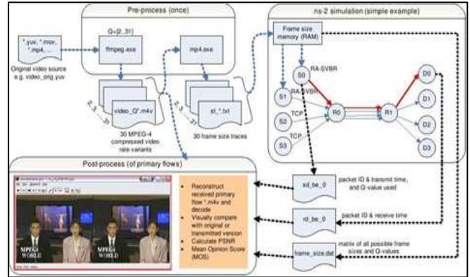
Fig. 1.2: simulation process of the Evalvid-RA framework [2]
