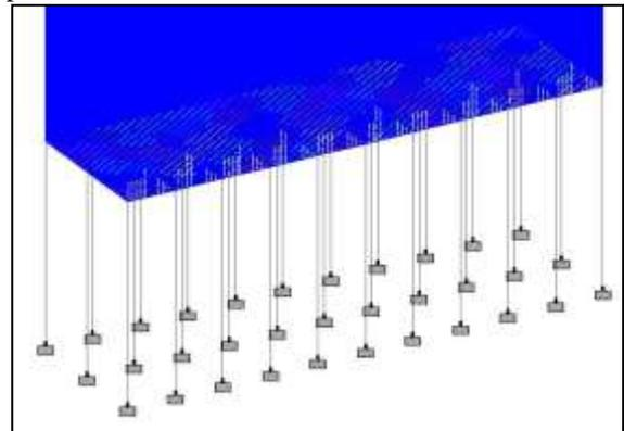
Fig. 2: Live load application in model
