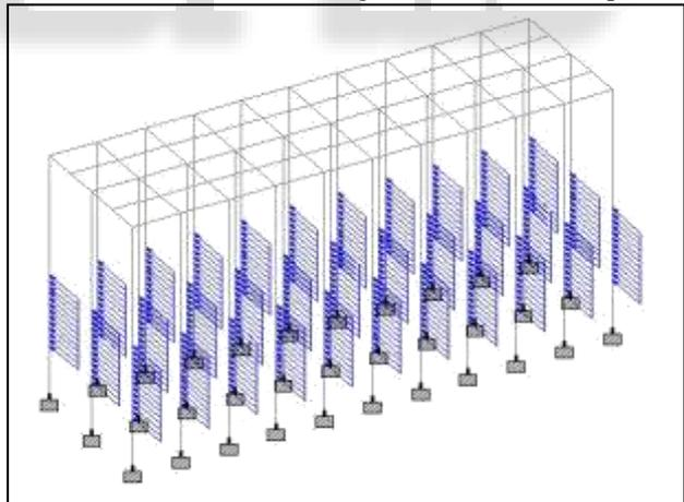
Fig. 6: Earth pressure application in model
