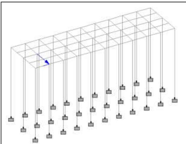
Fig. 8: Mooring force application in model
