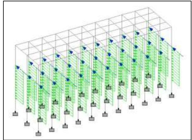
Fig 5: Current force and wave force application in model
