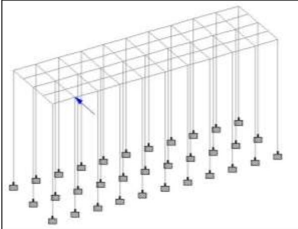
Fig. 7: Berthing force application in model
