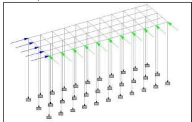
Fig. 3: Wind load applied model along X direction
