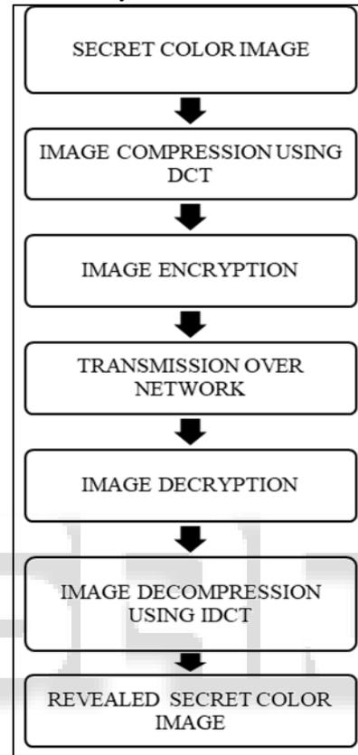
Fig. 3.1: Block Schematic of the proposed approach
