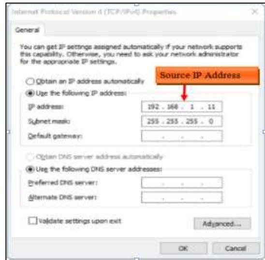
Fig. 7: Configuring the Laptop with manual IP address which is in the rule set
