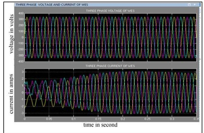
Fig. 7.3 3: phase Voltage and current of Wind Energy System
