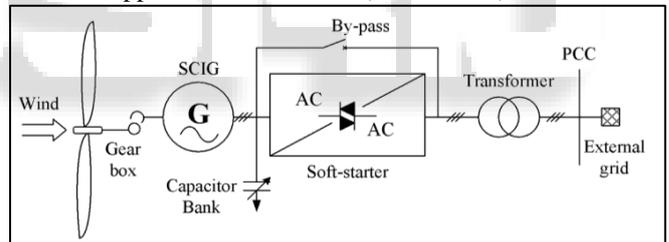
Fig. 3.5.1: Fixed-speed wind turbine with an induction generator.
