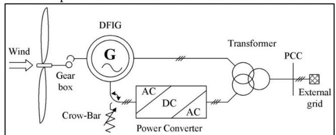
Fig. 3.5.2: Variable-speed wind turbine with a doubly-fed induction generator (DFIG)
