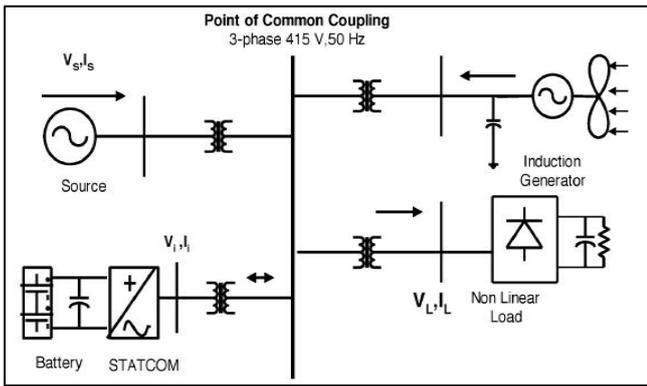
Fig. 5.1.1: Grid connected integrated wind energy system for power quality improvement
