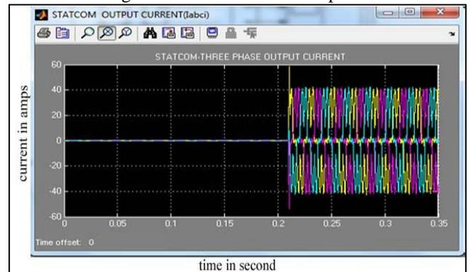
Fig. 7.5: Statcom Output Current
