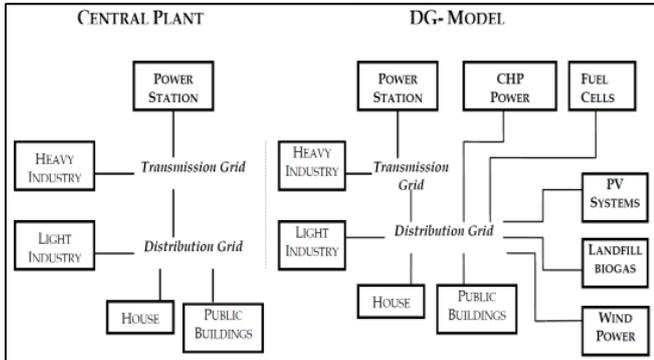
Fig. 4.0.1: Schematic diagram of traditionally central-plant model and DG-model
