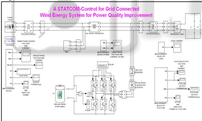
Fig. 5.2.2: Simulation model for STATCOM control
