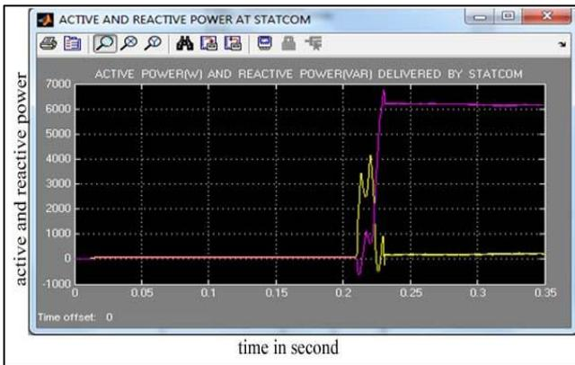
Fig. 7.6: Active (P) and Reactive Power (Q) in STATCOM
