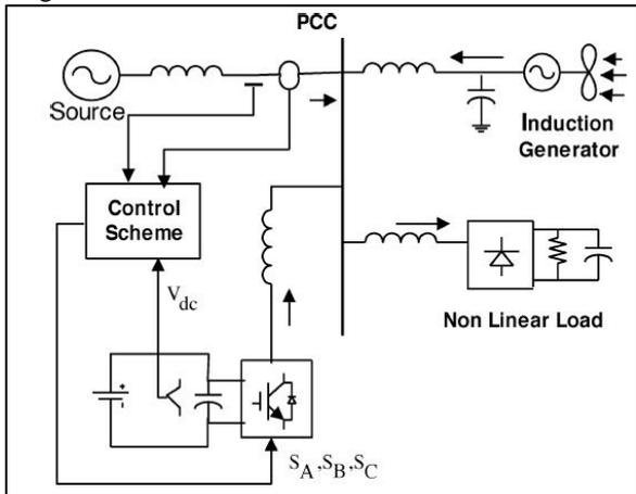
Fig. 5.2.3: control scheme with nonlinear load
