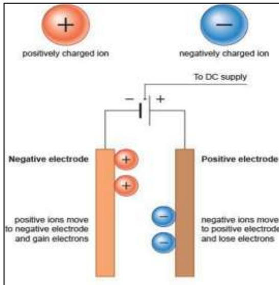
Fig. 1: Electrolysis process [2]
