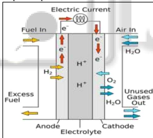
Fig. 2: Working of fuel cell [3]
