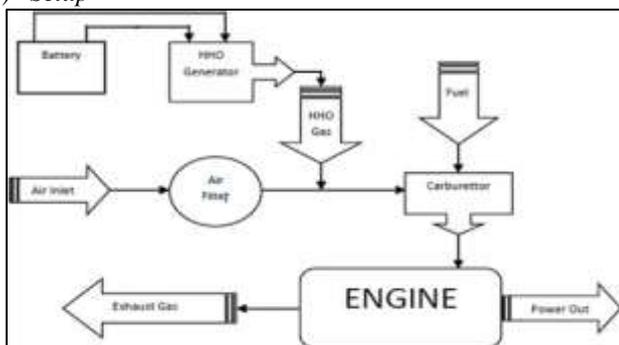
Fig. 3: schematic layout of installed HHO generation system on a vehicle or IC engine system [4]
