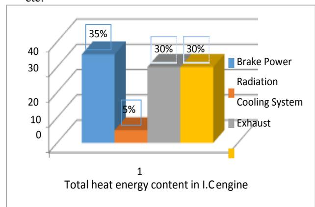
Fig. 1: show total energy distributions from internal combustion engine.
