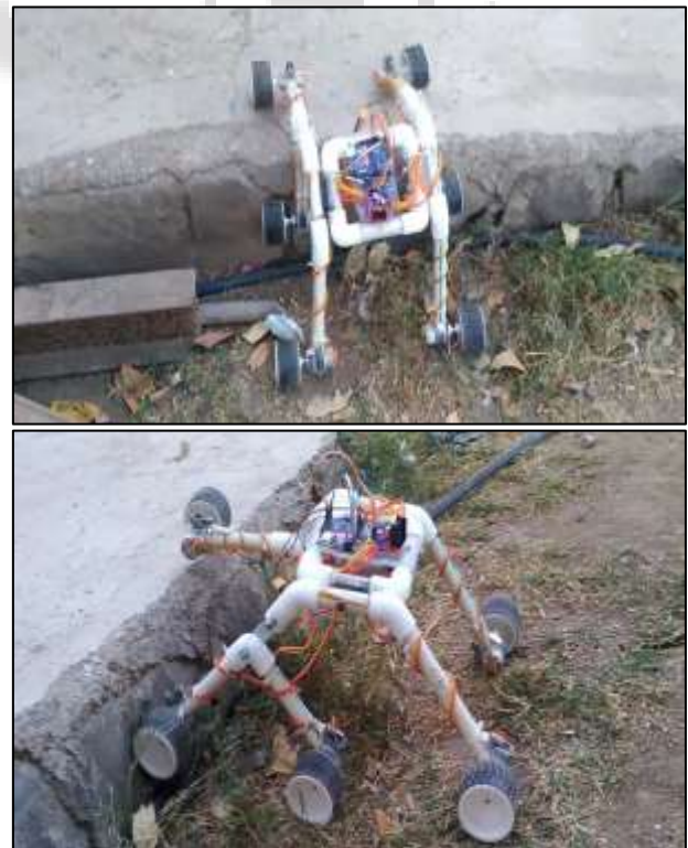
Fig. 1: The rocker bogie mechanism test on steps & off road area
