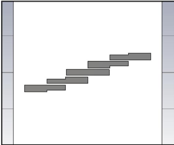
Fig. 1: coupled line band pass filter (middle layer).
