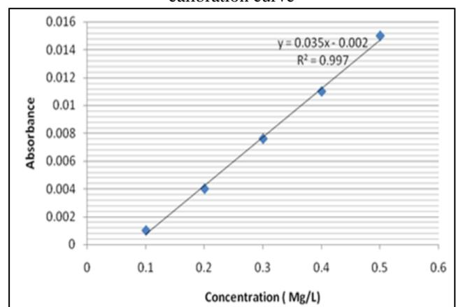
Fig. 3: Absorbance versus Concentration of Lead from calibration curve
