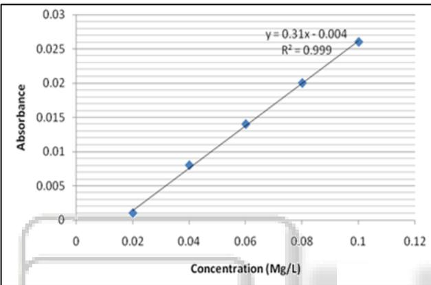
Fig. 5: Absorbance versus Concentration of Chromium from calibration curve
