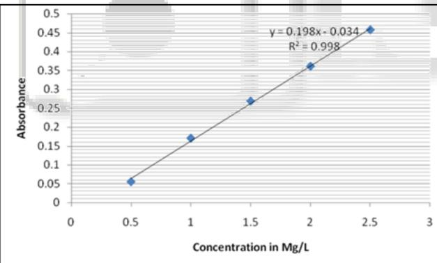
Fig. 6: Absorbance versus Concentration of Iron from Calibration curve
