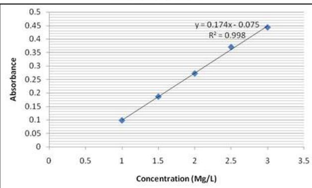
Fig. 7: Absorbance versus Concentration of Cobalt from Calibration curve
