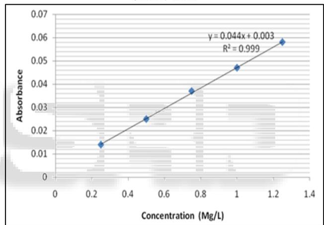
Fig. 2: Absorbance versus Concentration of Copper from calibration curve
