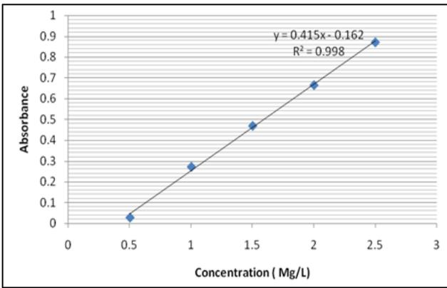
Fig. 4: Absorbance versus Concentration of Zin from calibration curve
