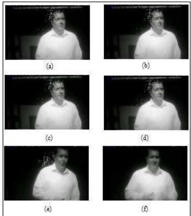
Fig. 7: system results using optical flow based on regular feature method (a) shows the first frame when detecting the face, and run the tracker, (b), (c), and (d) show the result of the tracker on some frames, (e) shows a false positive, and (f) shows a false negative.
