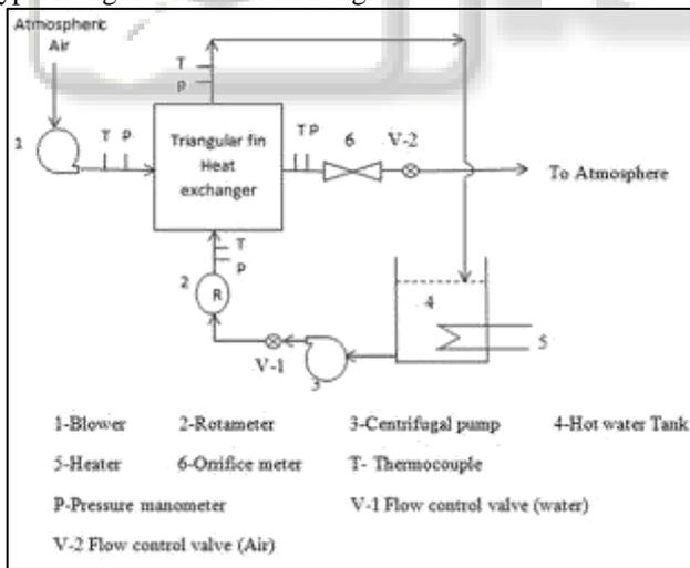
Fig. 2: Flow Diagram of Experimental set up
