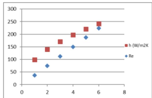
Fig. 3: Reynolds number (Re) vs. Heat transfer coefficient (h) at (55°C &  $q_{air} = 0.002132 \text{ m}^3/\text{s}$ )
