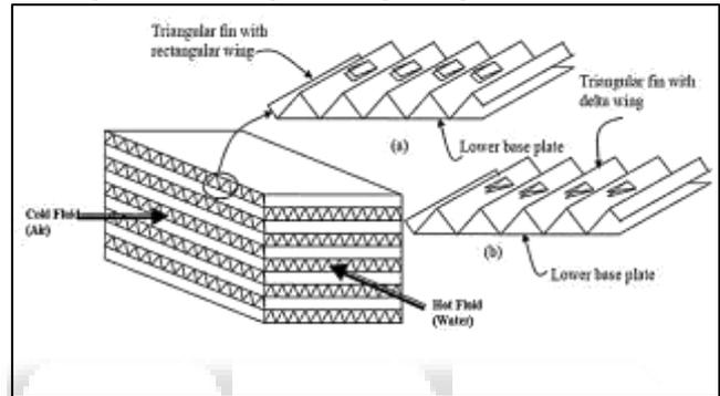
Fig. 1: Triangular Fin Heat Exchanger
