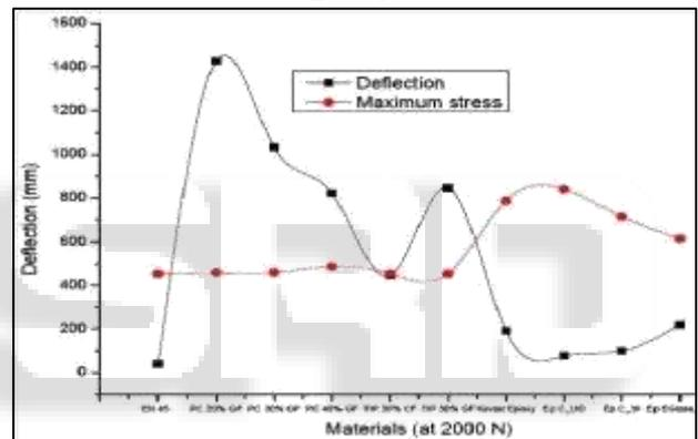
Fig. 6: Deflection (mm) & maximum stress (MPa) at 2000 N
