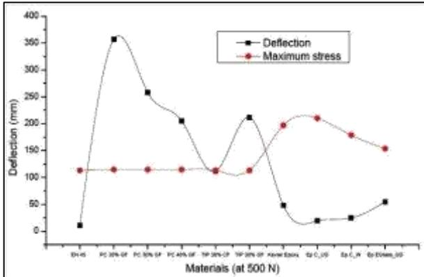
Fig. 4: Deflection (mm) and maximum stress (MPa) at 500N
