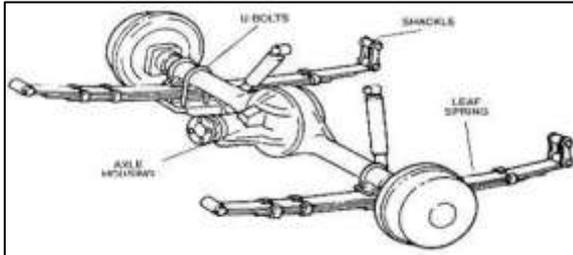
Fig. 1: Suspension System of automobile
