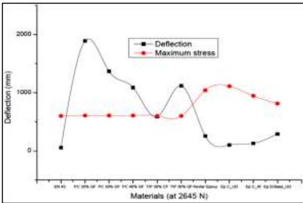
Fig. 7: Deflection (mm) & maximum stress (MPa) at 2645 N
