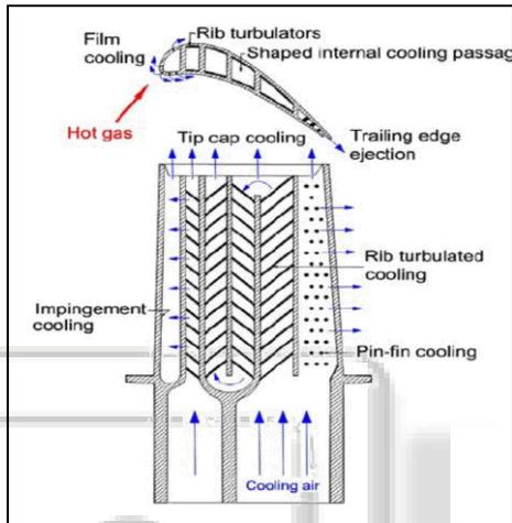
Fig. 1: Gas Turbine Cooling
