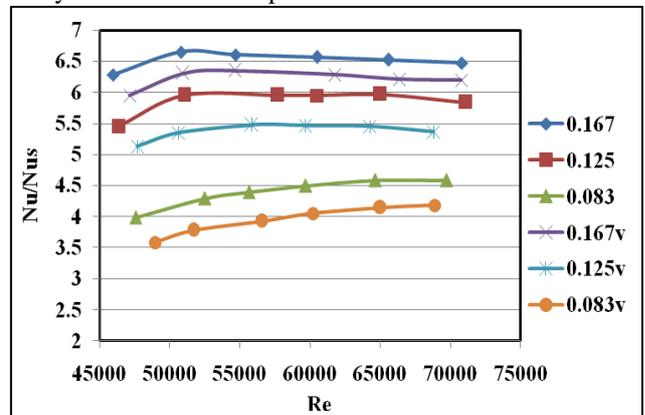
Fig. 8: Variation of Nusselt number ratio v/s Reynolds number for blockage ratio
