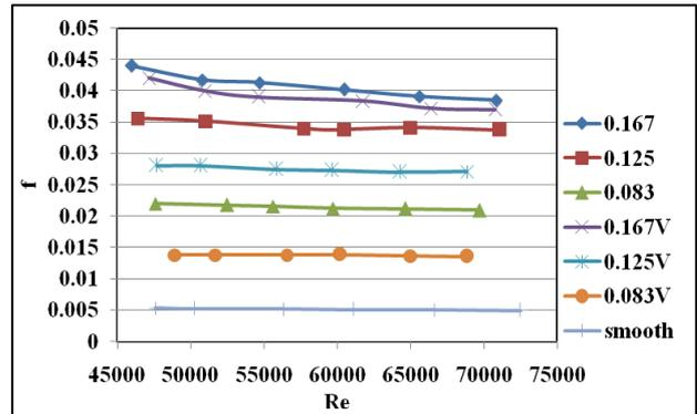
Fig. 7: Variation of Friction factor v/s Reynolds number for blockage ratio
