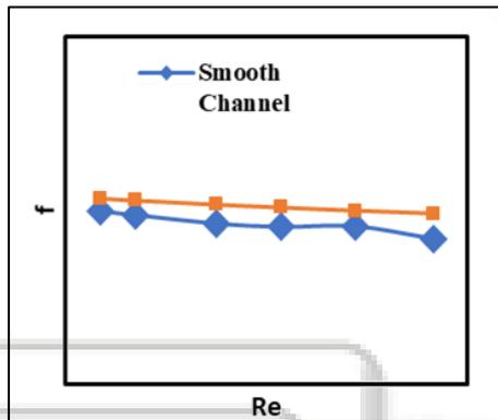
Fig.5 variation of friction factor v/s Reynolds number for smooth duct
