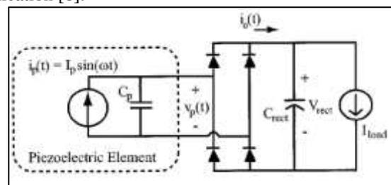
Fig. 7: Piezoelectric element model with ac-dc rectifier and load
