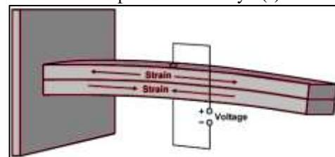
Fig. 6: Cantilevered beam with piezoceramic layers.
