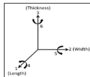
Fig. 4: Piezoelectric axes
