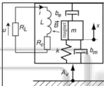
Fig. 2: Example of an electromagnetic energy harvesting
