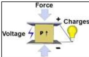
Fig. 1: Example of an electromechanical energy harvesting
