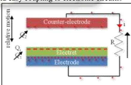
Fig. 3: Example of an electrostatic energy harvesting
