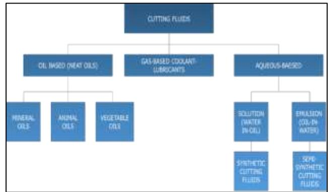
Fig. 2: Classification of cutting fluids
