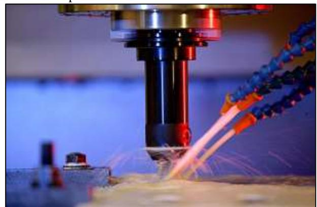
Fig. 1: Metal Cutting Fluid
