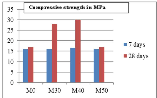
Fig. 1: Effect of cement replacement by UFFA on Compressive strength of 1:3 mortar
