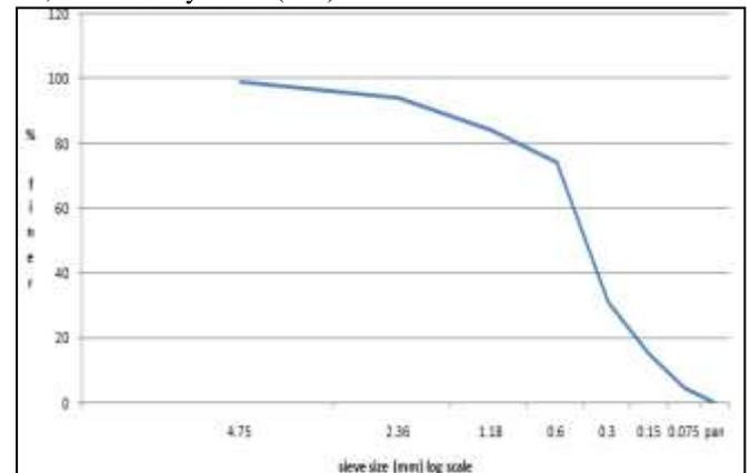
Graph 1: % finer vs sieve size in mm (log scale)
