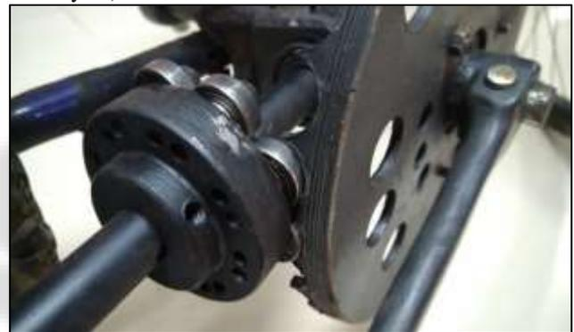
Fig. 2: Bearings Enclosure with Sprocket
