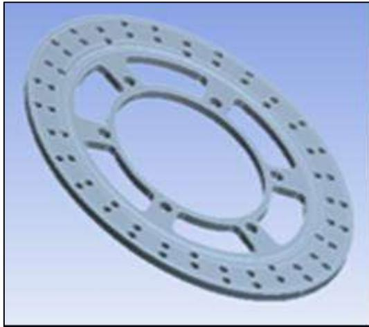
Fig. 2: New Disc brake 3D Model
