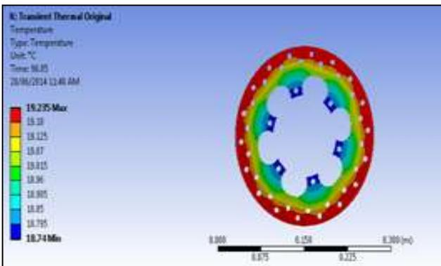
Fig. 3: Transient Thermal Analysis Result- Selected Disc (sample disc 1)
