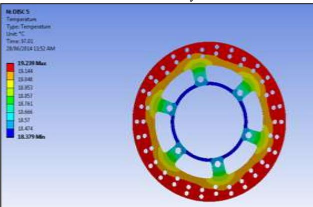
Fig. 4: Transient Thermal Analysis Result (ANSYS) of New Disc
