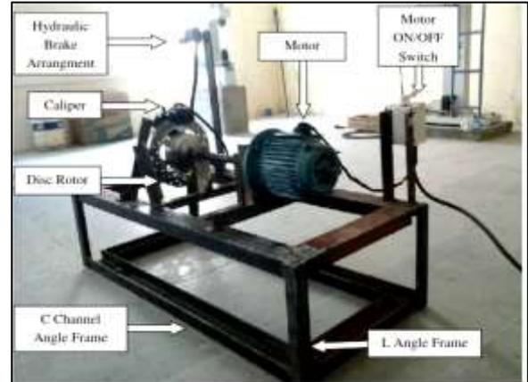
Fig. 5: Experimentation Setup
