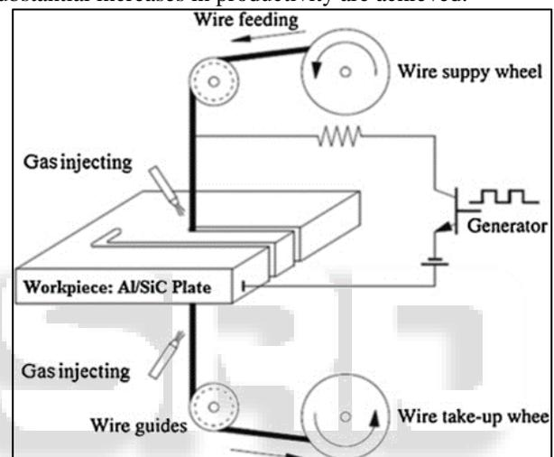
Fig.1 (a): Schematic of WEDM Process
