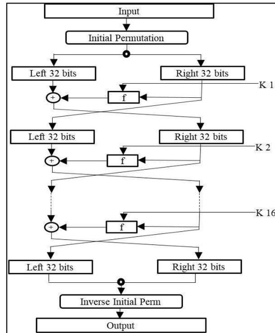
Fig. 2.2: Data Encryption Standard Process
