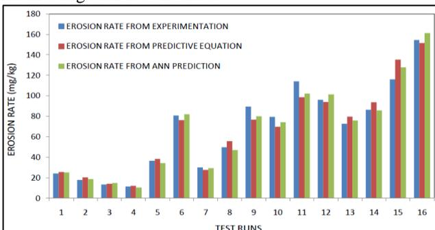
Fig. 3.4: Comparison of Erosion Rates Obtained from Different Methods
