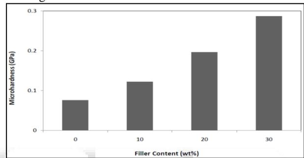
Fig. 3.1: Micro-Hardness of Blast Furnace Slag filled Composites
