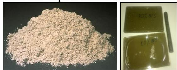
Fig. 2.1: Blast Furnace Slag & Composite Samples
