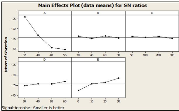
Fig. 3.2: Effect of Control Factors on Erosion Rate for Polyester-BFS Composites
