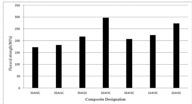
Fig. 2: Effect of flexural strength on SiC and Co powder filled Al 6061 Composites
