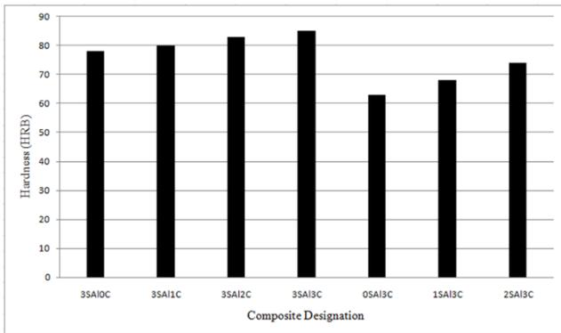
Fig. 1: Effect of hardness on SiC and Co powder filled Al 6061 Composites
