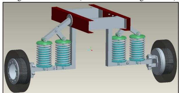
Fig. 1: Independent Front Wheel Suspension Unit Assembly
