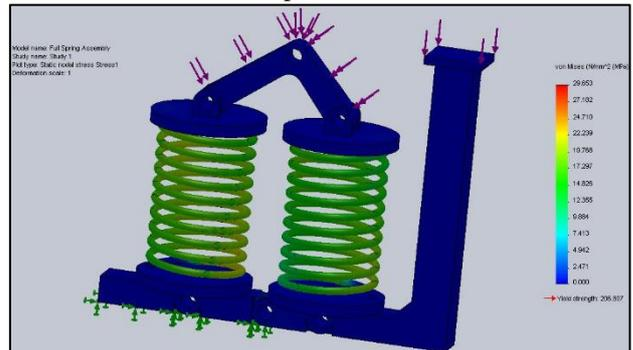
Fig. 11: Spring Assembly Analysis Mode 5: Static Nodal Stress
