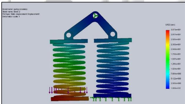
Fig. 8: Spring Assembly Analysis Mode 2: Static Displacement
