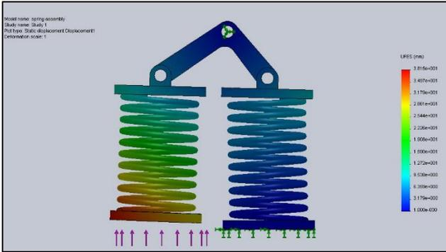
Fig. 6: Spring Assembly Analysis Mode 1: Static Displacement
