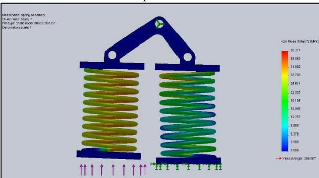
Fig. 7: Spring Assembly Analysis Mode 1: Static Nodal Stress
