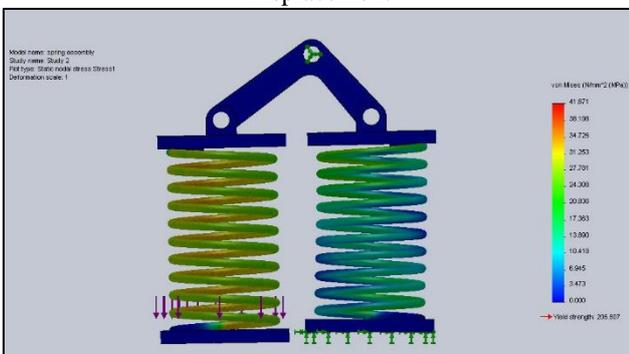
Fig. 9: Spring Assembly Analysis Mode 2: Static Nodal Stress
