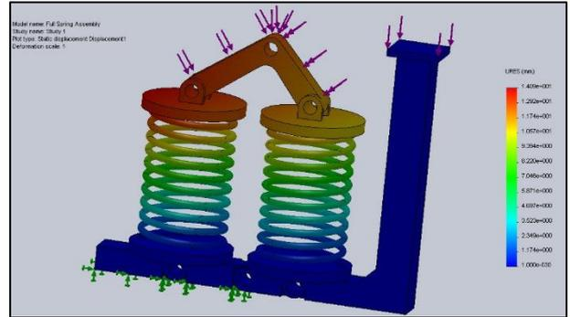
Fig. 10: Spring Assembly Analysis Mode 5: Static Displacement
