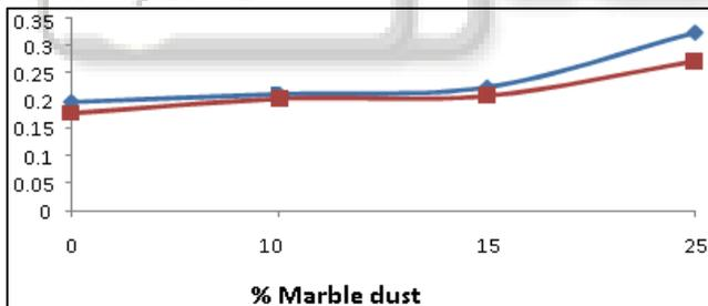
Fig. 6: Abrasion Resistance of Concrete Paving Blocks Containing Marble Dust for Varied w/c Ratio
