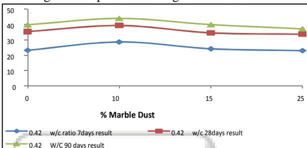
Fig. 5: Compressive Strength at w/c ratio 0.42
