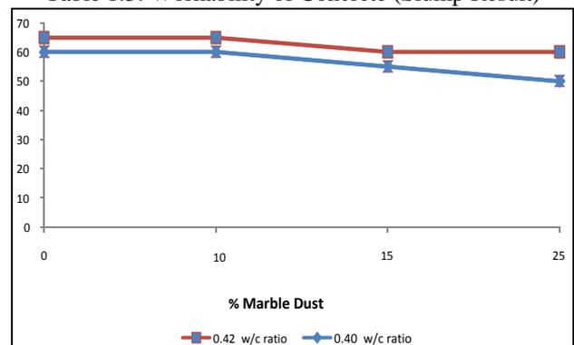
Fig. 3: Slump Value of Different Concrete Mix
