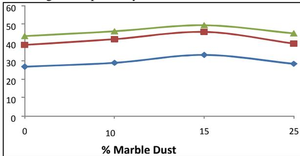
Fig. 4: Compressive Strength at w/c ratio 0.40
