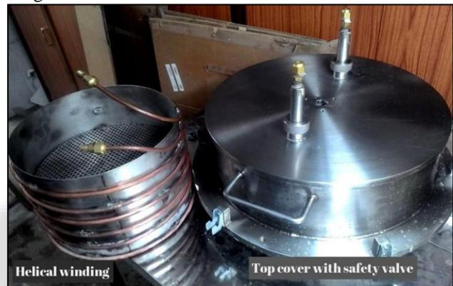
Fig. 1: Vessel for Cryotreatment
