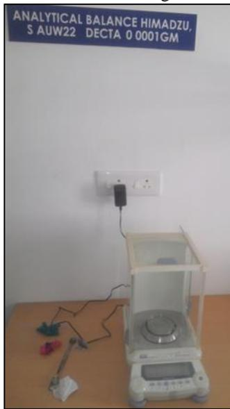
Fig. 3: Analytical Balance for Mass Measurement
