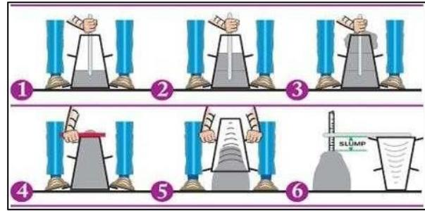
Fig. 1: Concrete Slump Test Procedure
