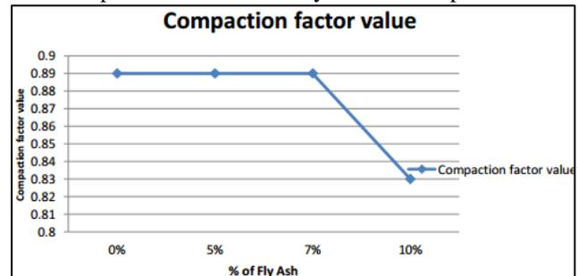
Graph 2: Indicates % of flyash vs Compaction factor
