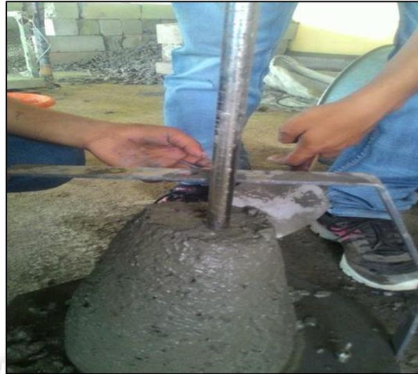
Fig. 2: Slump Cone Test at Site
