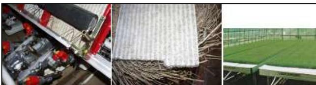
Fig. 1: (Left) Japanese Trans planter Adapted to take a seed mat, (center) seed mat with rice seeds and fertilizer embedded in card (Right) Rice Seedling Ready for Transplanting
