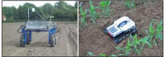
Fig. 2: (Left) Portal crop scouting platform (Madsen and Jakobsen 2001), (Right) Sub Canopy robot ISAAC2 built by a student team Hohenheim University ([www.fieldrobot.nl](http://www.fieldrobot.nl))
